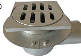
Special duty solid cover with perimeter drain gap (-PD) (Grate part # - P3080-PG-PD)
